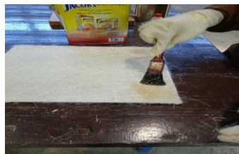
Figure 4: The process of coating a resin mixture on glass fibers
