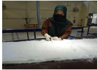
Figure 3: The process of cutting fiberglass mats
