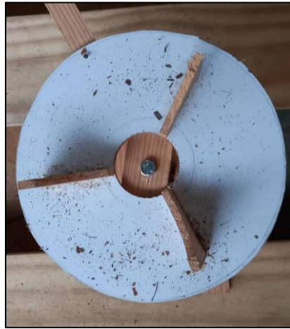
Figure 10: Wheel and axle on the coconut holder
