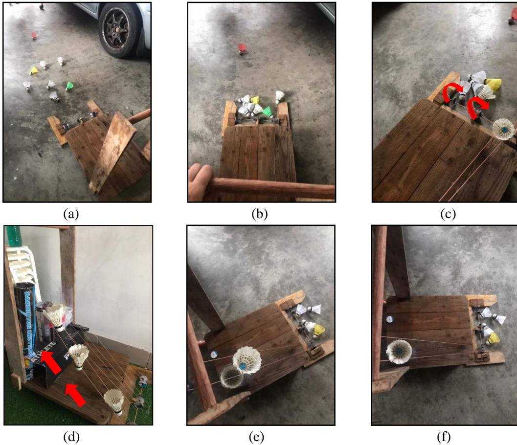
Figure 7: Process of collecting shuttlecock using Shuttlecock Collector Machine
