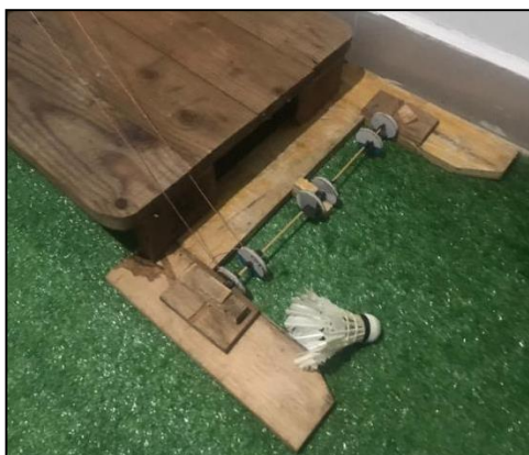
Figure 13: Shuttlecock stuck under sweeper
