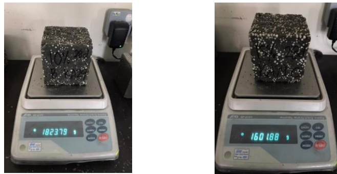
Figure 3 (a) 10% of Replacement Concrete Figure 3 (b) 15% of Replacement Concrete
