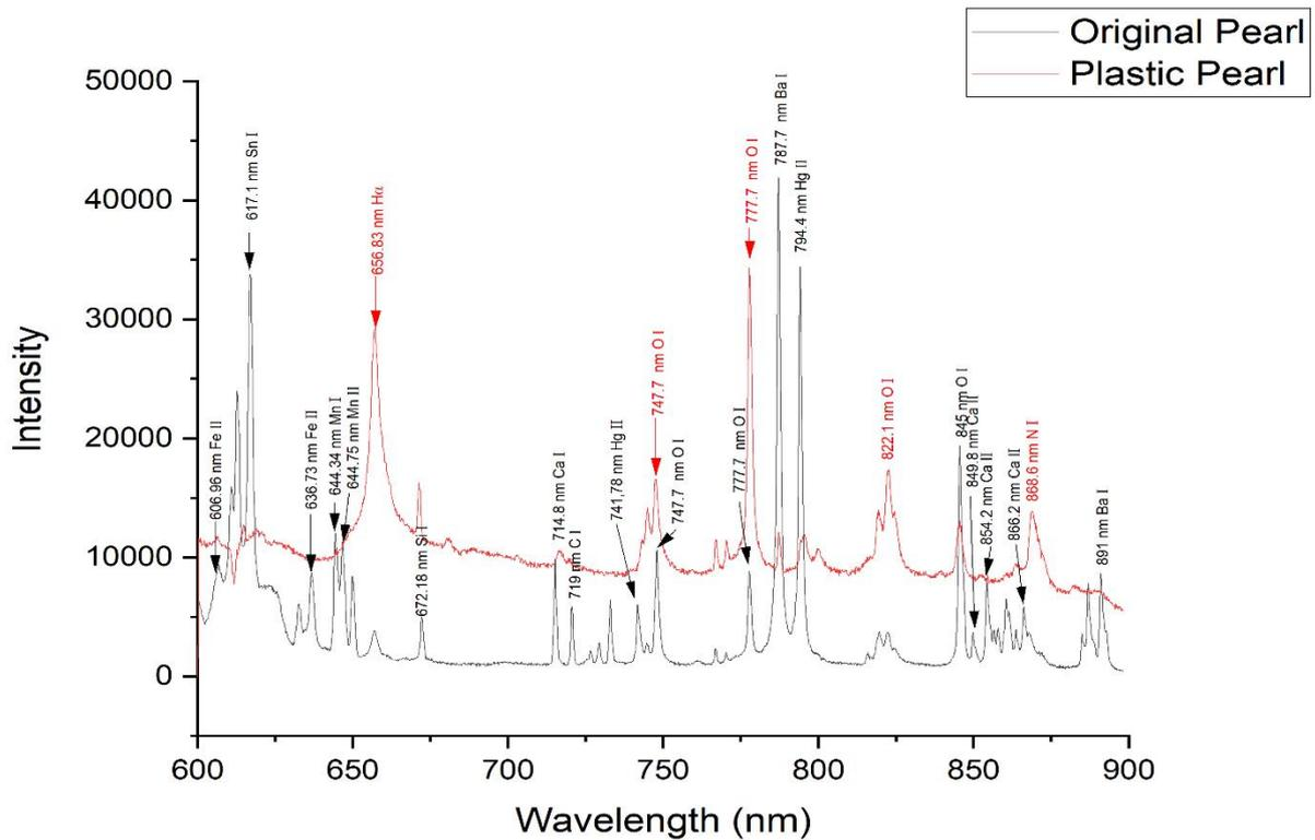
Figure 2: Emission spectrum obtained by laser ablation on original pearl and plastic one
