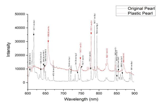
Figure 2: Emission spectrum obtained by laser ablation on original pearl and plastic one
