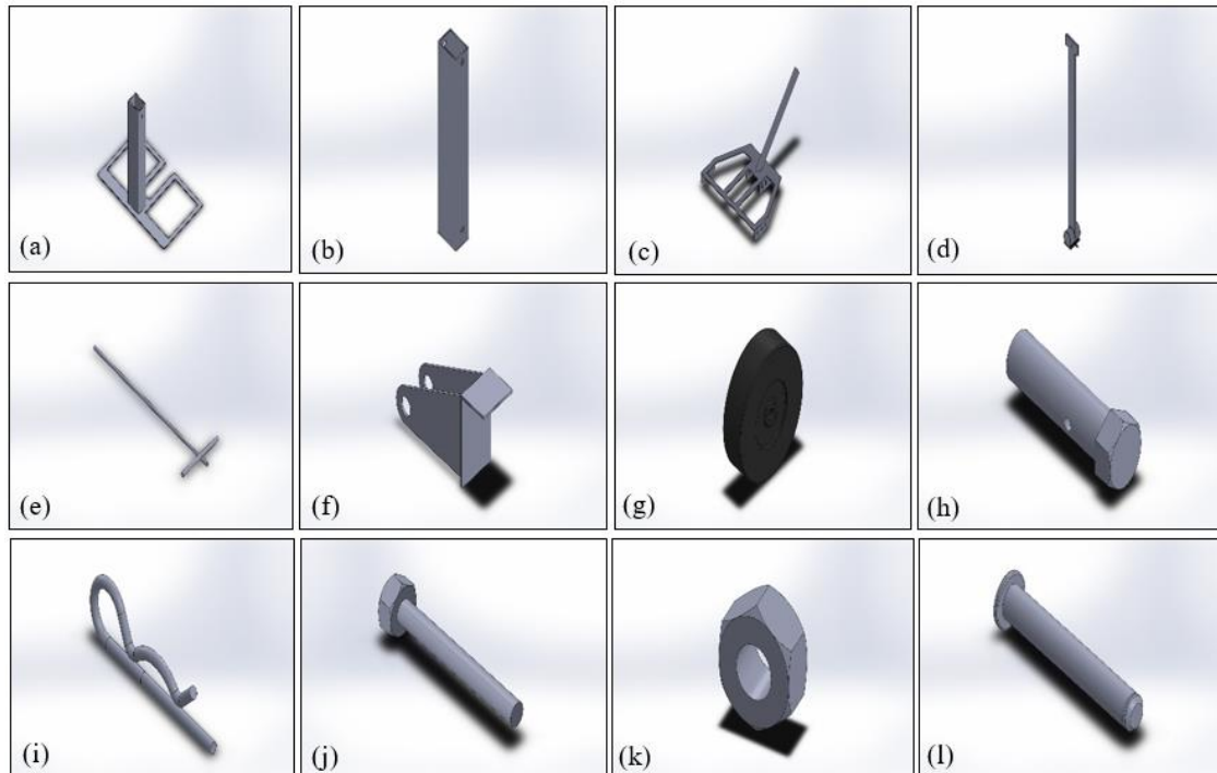
Figure 1: Part design using SolidWorks 2019 software, (a) Base, (b) Vertical, (c) Presser, (d) Handle, (e) Cylinder handle, (f) support, (g) Wheel, (h) Bolt size 30 mm × 10 mm (i) Pin, (j) Bolt size 90 mm × 10 mm, (k) Shaft, (l) Pin slot
