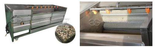
Figure 1: Oyster Cleaning Machine and its brush [7]
