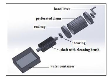
Figure 6: Exploded Design of Cockle Cleaning Machine
