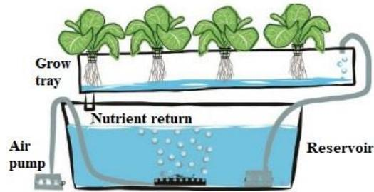
**Figure 1: NFT Hydroponic system.**
