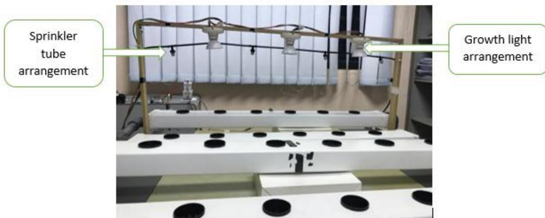
**Figure 8: Complete controlled hydroponic system arrangements.**
