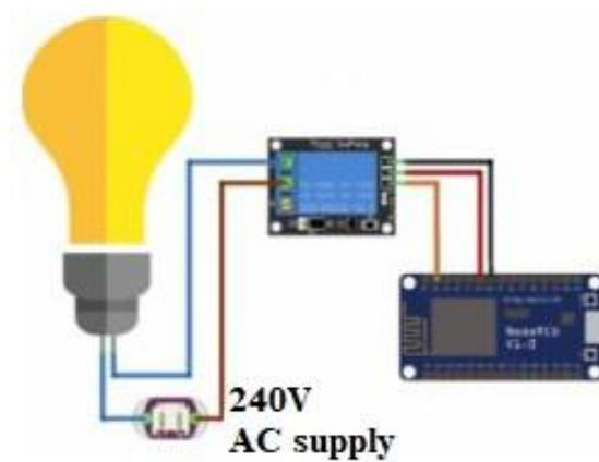
Figure 6: Growth light connection with relay and NodeMCU
