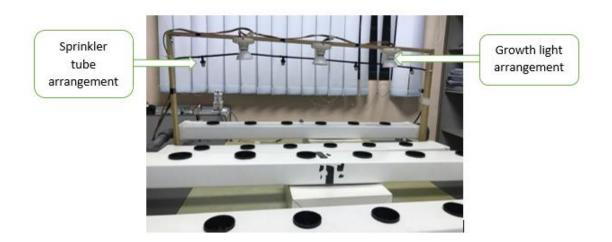
Figure 8: Complete controlled hydroponic system arrangements.
