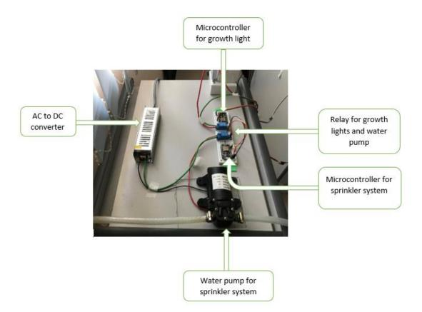
Figure 7: Complete component arrangement for the controlled system.
