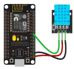
Figure 5: Pin connection between NodeMCU and DHT11 sensor.
