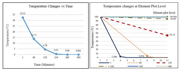
Figure 6: Temperature Changes vs Time Figure 7: Temperature changes at the elements plot level
