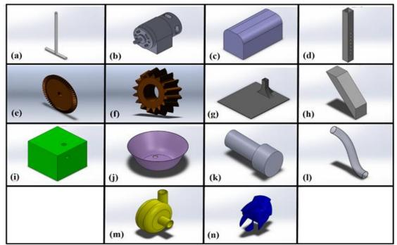
Figure 3: Machine parts by Solid Work 2019 (a)spreader, (b) DC motor, (c) Casing, (d) Square bar, (e) Bevel gear, (f) Pinion bevel gear, (g) Base, (h) Support rib, (i) Frame, (j)Bowl, (k) Fastening pin, Transferring tube, (m) Centrifugal pump, (n)Impeller fan
