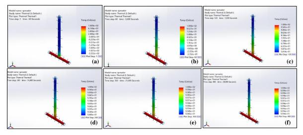
Figure 5: Thermal transient FEA analysis of image profile for 100°C heating up on pan in a different time, (a) 1 minute, (b) 1 hour, (c) 2 hours, (d) 4 hours, (e) 6 hours, (f) 8 hours
