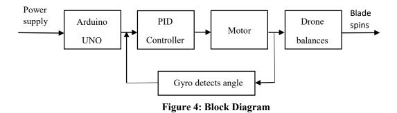
**Figure 4** is the configuration of block diagram of dualcopter. It is a closed loop control system because it has feedback. The input is power supply and the error detector is Arduino UNO. PID controller is the controller and motor are the actuating signal. The plant is drone balances and the output is blade spins. Gyro detects angle is the feedback of this system.
