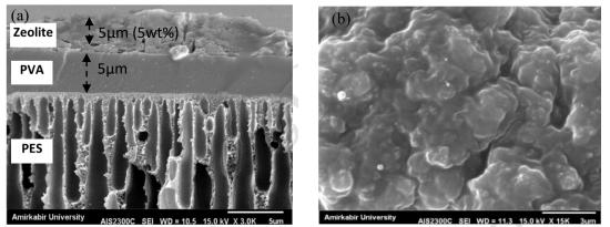
Figure 2: (a) The cross section and (b) top surface of multi-layer nano zeolite X/PVA/PES membrane [22]
