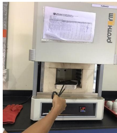
Figure 5: Furnace used in drying process
