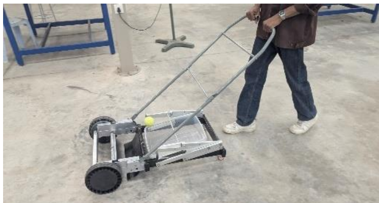
Fig. 4 Prototype performance test for foldable tennis ball picker
