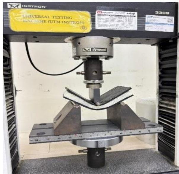
Fig. 4 Flexural testing is being tested on sandwich panels
