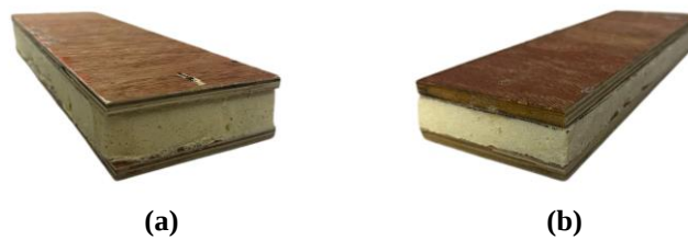
Fig. 2 Design for Sandwich Panel (a) Model thickness 5 cm; (b) Model thickness 3.4 cm
