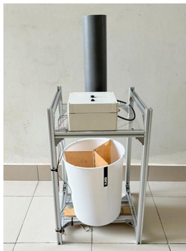
Fig. 3 The Sound Activated Sorting Bin Model
