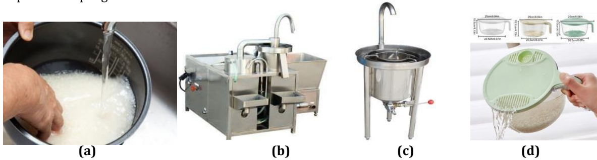
Rajah 1 Proses Mencuci Beras (a) Secara manual; (b) Mesin Mencuci Beras TM-600 [5]; (c) Rice Bean Washer RW-25 [5]; (d) Portable Rice Cleaning Bowl
