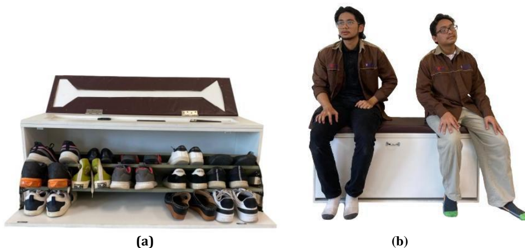
Fig 5 Test Run for the Multi-Level Shoe Rack (a) 12 pairs of various shoes; (b) 2 adults sit on the shoe rack
