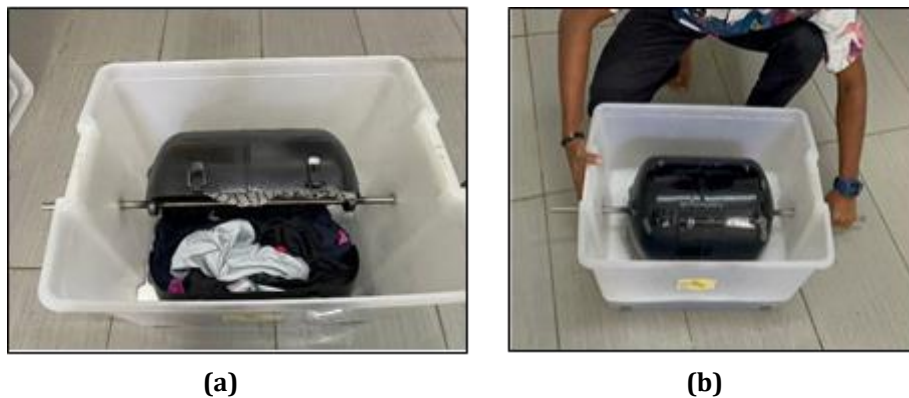
Fig. 3 Testing on washing machine (a) Putting all the clothes inside the drum; (b) Spin the machine manually
