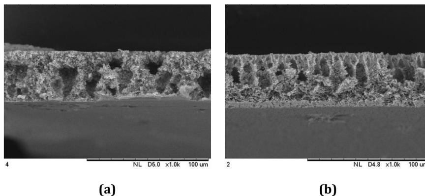
**Fig. 3** SEM images cross section flat sheet membrane for ratio (a) 0:10; (b) 9:1
