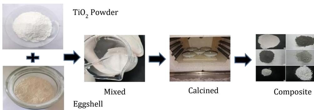
**Fig. 1** Preparation of eggshell/TiO<sub>2</sub> composite for each ratio
