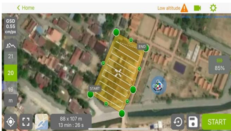
Fig.1 Area set before UAV flight using Pix4D Capture
