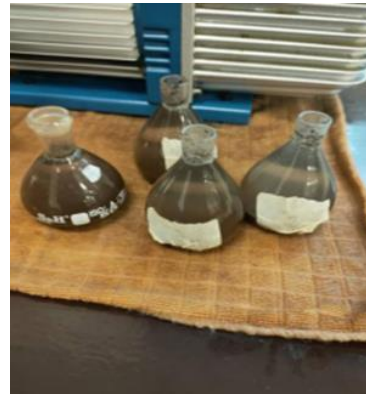
Fig. 4 Specific gravity test. (a) Vacuum pump, (b) Distilled water with sample in a volumetric flask
