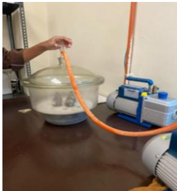
Fig. 4 Specific gravity test. (a) Vacuum pump, (b) Distilled water with sample in a volumetric flask
