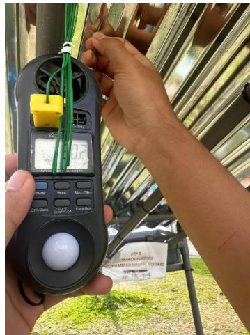
Fig. 5 Temperature Testing of Cooling System
