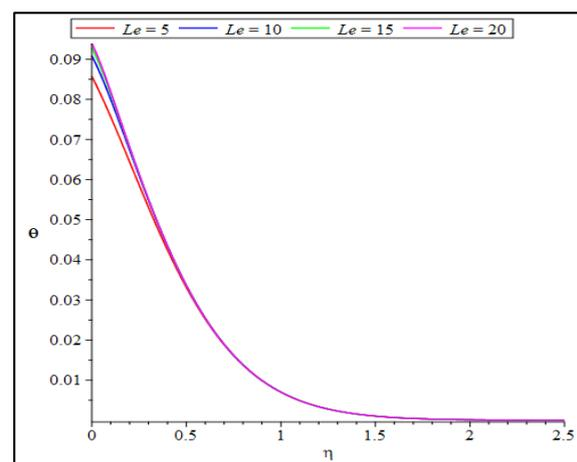
**Figure 3: Effect of  $Le$  on temperature**
