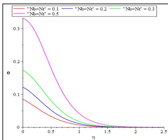
**Figure 2: Effect of  $Nt$  and  $Nb$  on temperature**
