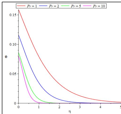
**Figure 5: Effect of  $Pr$  on temperature**
