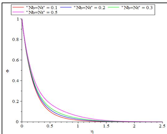
**Figure 6: Effect of  $Nt$  and  $Nb$  on concentration**
