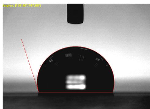
**Figure 14: an image of water contact angle of S Nano hydrophobic liquid repellent for four (4) layers of coatings.**
