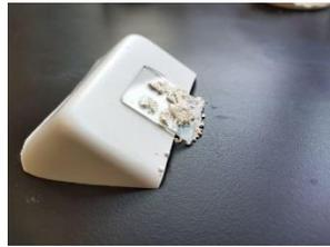
**Figure 15: an image of glass slide coated with DPRO super hydrophobic glass coating**
