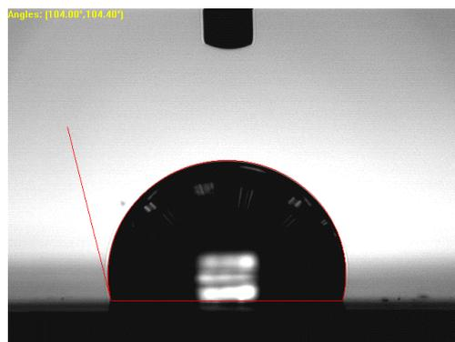
**Figure 13: an image of water contact angle of DPRO super hydrophobic glass coating for four (4) layers of coatings.**
