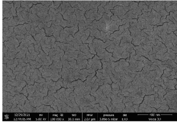
**Figure 4: a surface morphology of DPRO super hydrophobic glass coating 100000x of magnification**
