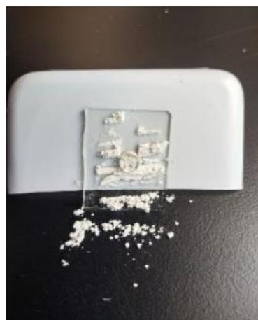
**Figure 11: an image of glass slide coated with S Nano hydrophobic liquid repellent**
