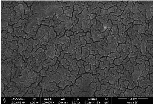
**Figure 3: a surface morphology of S Nano hydrophobic liquid repellent at 100000x of magnification**
