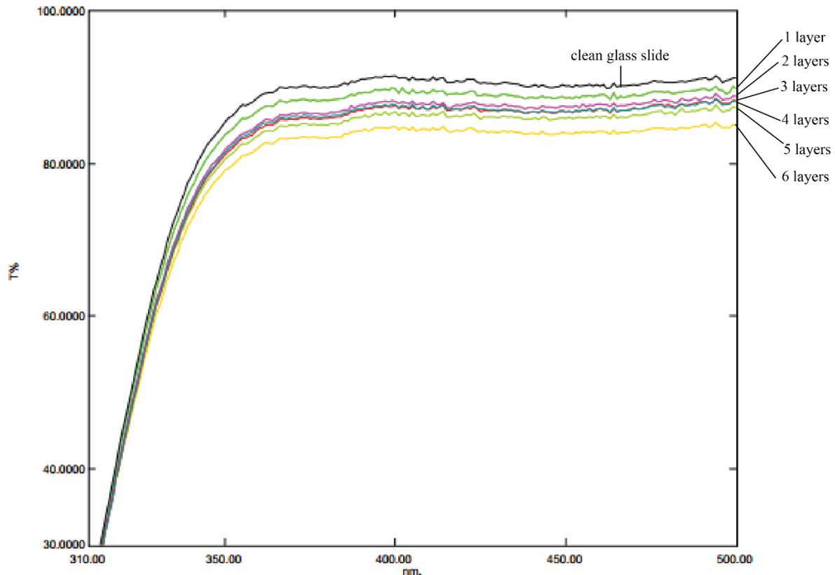
**Figure 2: UV-Vis spectrophotometer results for S Nano Hydrophobic Liquid Repellent solutions' coated glass slides.**
