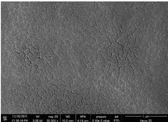
**Figure 5: a surface morphology of S Nano hydrophobic liquid repellent at 50 000x of magnification.**
