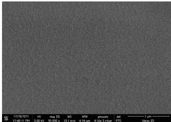
**Figure 6: a surface morphology of DPRO super hydrophobic glass coating at 50 000x of magnification.**
