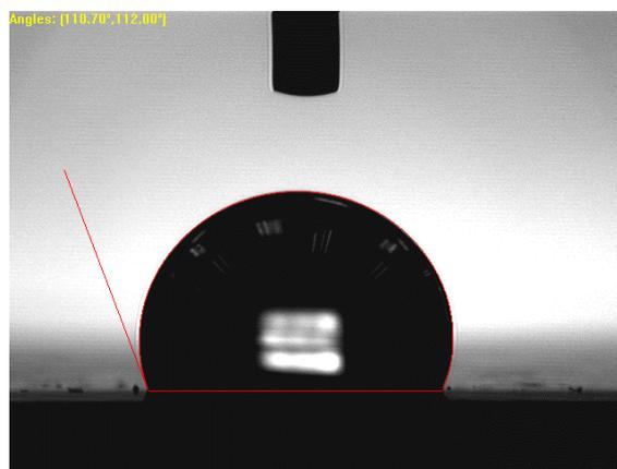
**Figure :8** an image of water contact angle for S Nano hydrophobic liquid repellent for four (4) layers of coatings.
