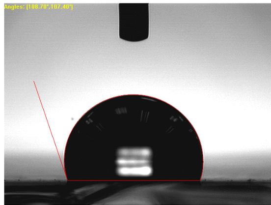
**Figure 7:** an image of water contact angle of DPRO super hydrophobic glass coating for four (4) layers of coatings.
