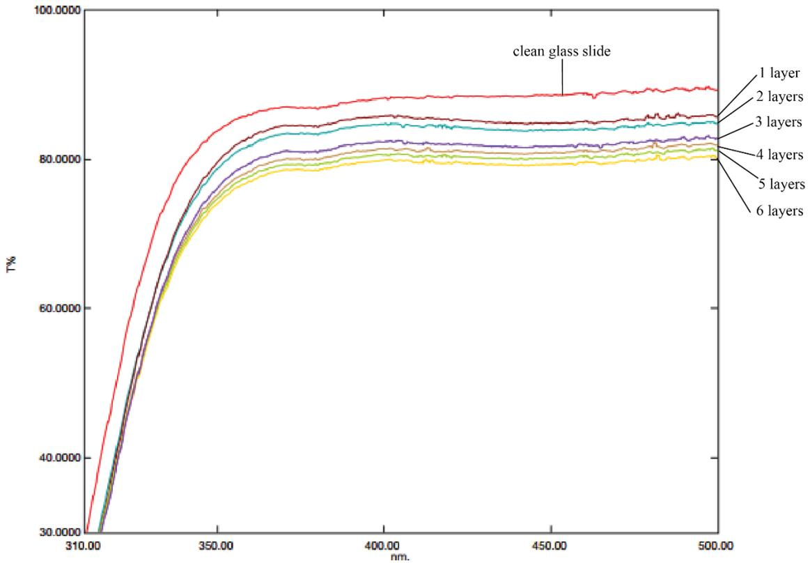
**Figure 1: UV-Vis spectrophotometer results for DPR0 Super Hydrophobic Glass Coating Ceramic Window Coating solutions' coated glass slides.**
