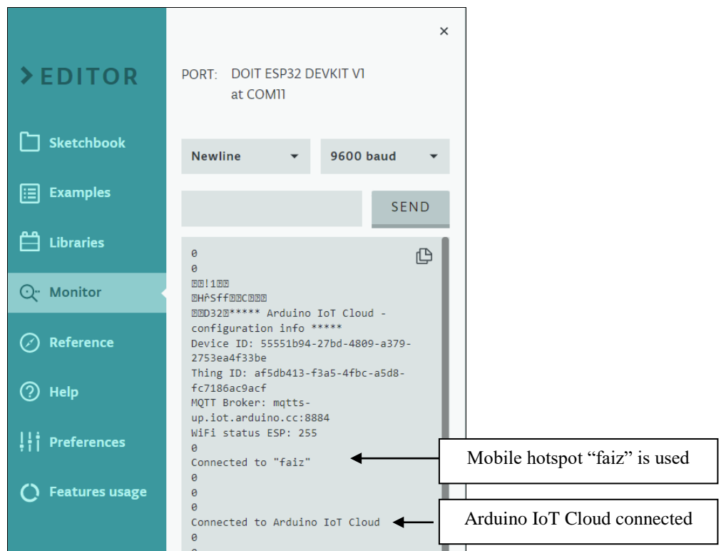
Figure 5: Serial monitor of Arduino IoT Cloud.
