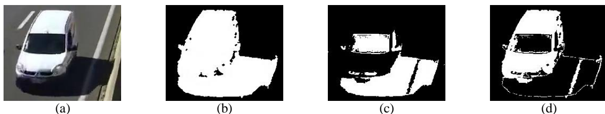
Fig. 3 (a) Original frame; (b) Detected foreground; (c) Binary map of shadow region; (d) Binary map after shadow removal
