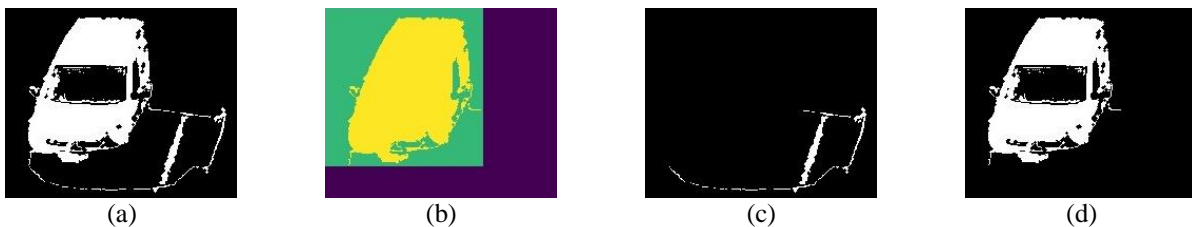
Fig. 4 (a) Binary map after shadow removal; (b) Segmentation with Graph Cuts; (c) Shadow region extracted with Graph Cuts; (d) Binary map after shadow removal with Graph Cuts
