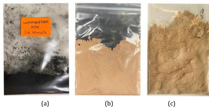
Fig. 1 The samples of POFA which are (a) untreated POFA (UTPOFA), (b) heat treated POFA (HTPOFA), and (c) chemically treated POFA (CTPOFA)
