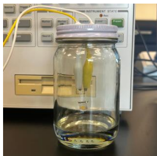
Fig. 6 QCM sensor testing in closed container
