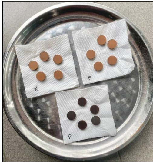
Fig. 4 Pellets with additives were dried under sunlight for 6 hours to reach absorption equilibrium
