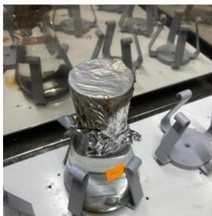
Fig. 2.1 Immersion test set up inside the shaker incubator at a constant temperature.
