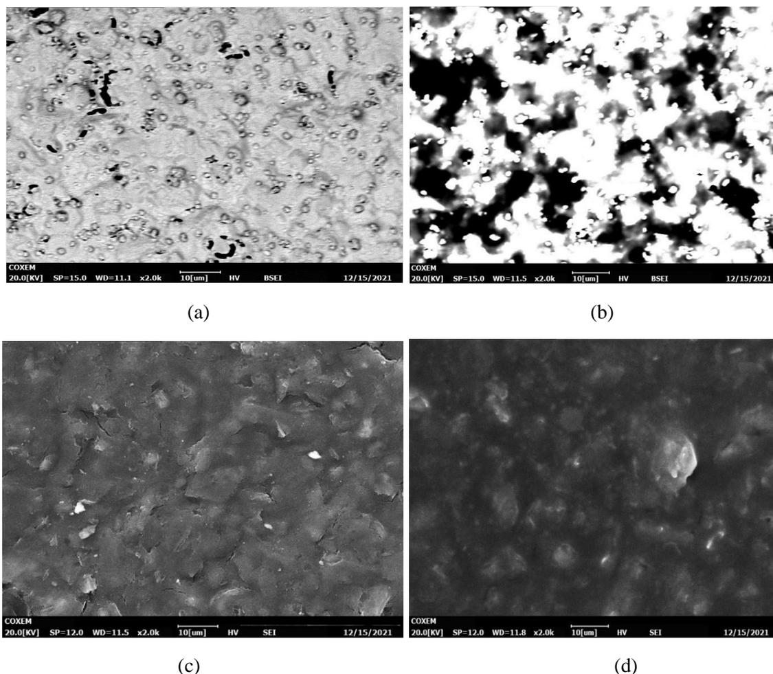
**Figure 4: (a) Gold SPE before immobilization; (b) Gold SPE after immobilization; (c) Carbon SPE before immobilization; (d) Carbon SPE after immobilization**
