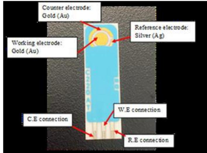
Figure 5: Dropsens gold screen-printed electrode (SPE)
