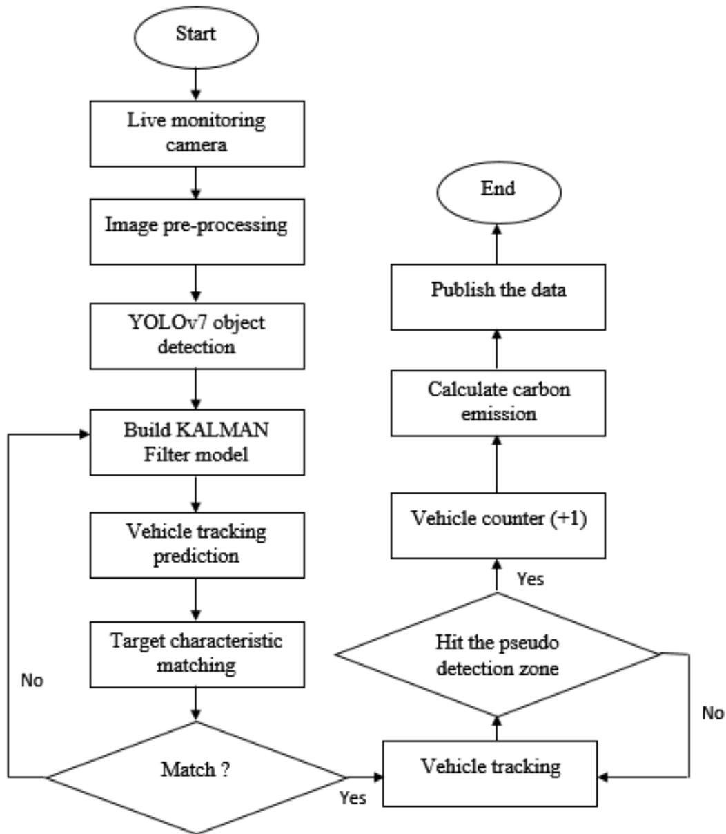
Figure 1: The flow chart for type of vehicle recognition system.
