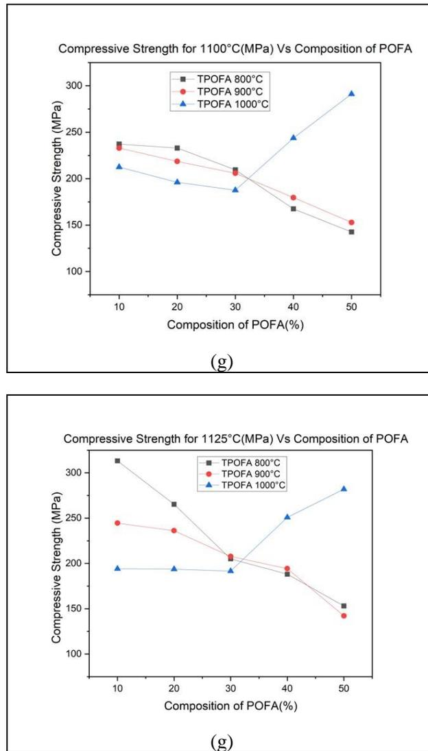
**Figure 4: Compressive Strength for (g) 1100 °C (h) 1125 °C**
