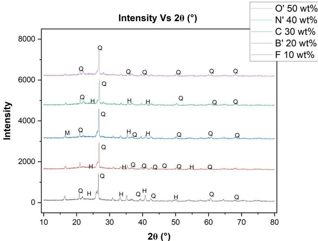
Figure 6: The XRD of clay-POFA samples.
