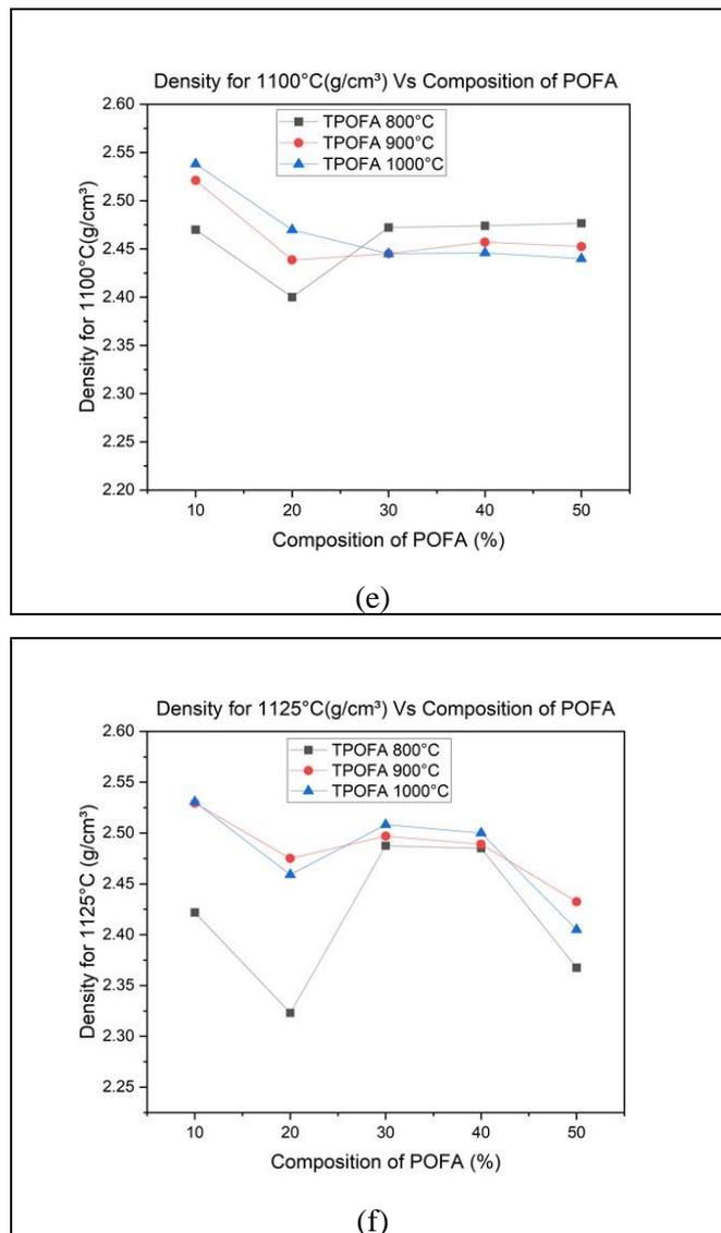
**Figure 3: Graph Bulk Density for (e) 1100 °C (f) 1125 °C**
