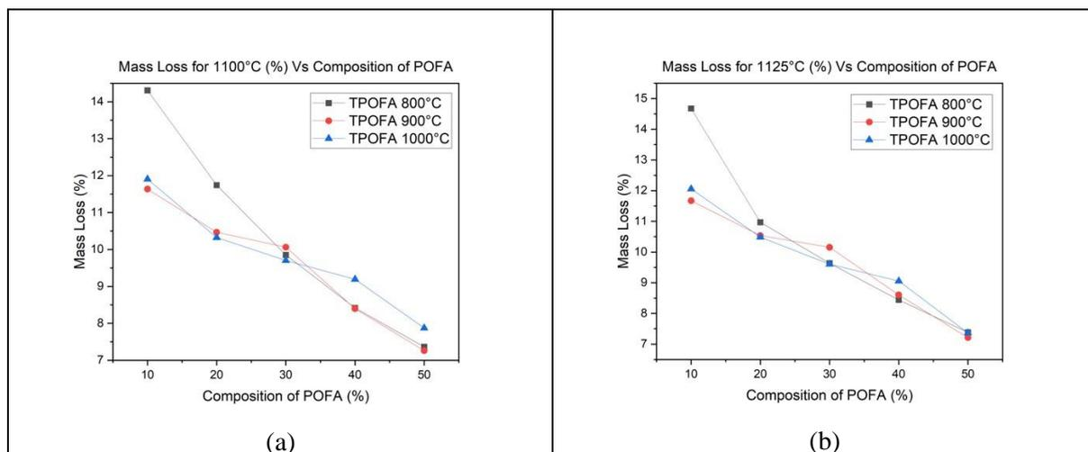
**Figure 1: Graph of Mass Loss for (a) 1100 °C and 1125 °C**
