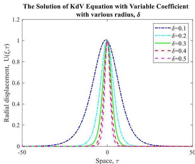
Figure 2: Radial displacement,  $U(\xi, \tau)$  versus space,  $\tau$  with various radius,  $\delta$  at  $-50 \leq \tau \leq 50$
