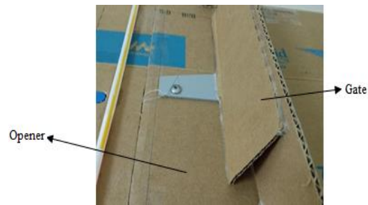
Figure 9: 'Gate' and 'opener' structures on physical segregation mechanism
