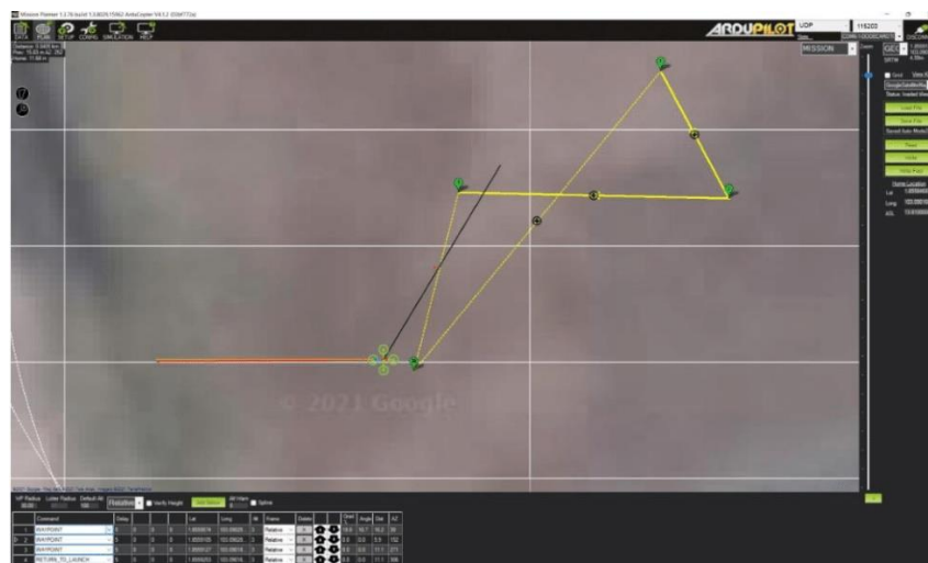
Figure 3: The waypoints for the UGV when moving using GPS navigation
