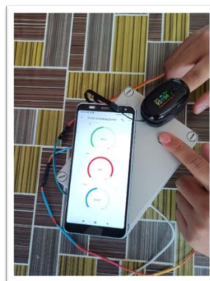
Figure 4: Prototype Pulse Rate Test
