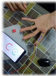
Figure 7: Prototype testing of the flex sensor
