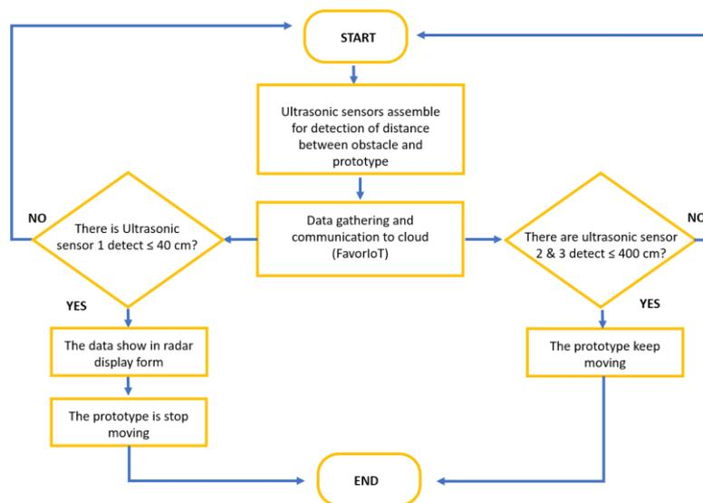
Figure 2: Flowchart the railway obstacle detector system
