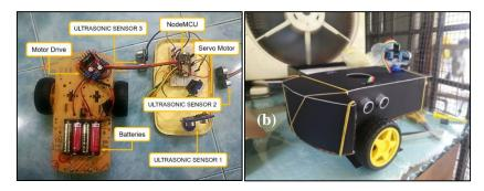
Figure 3: (a) Arrangement of circuit and (b) final prototype
