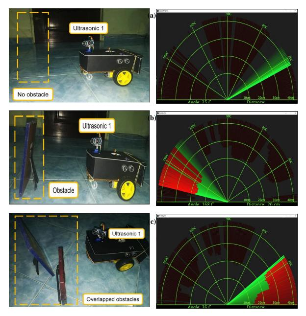
Figure 4: Three testing with (a) "no obstacle", (b) "obstacle" and (c) "overlapped obstacles" conditions with respective radar displays.
