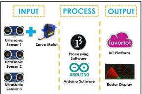
Figure 1: The block diagram of an obstacles detection system
