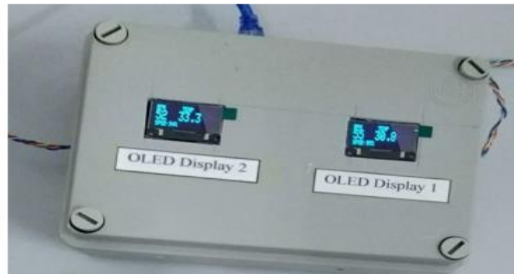
Figure 10: OLED Display showing the SpO 2 , BPM, and Body temperature
