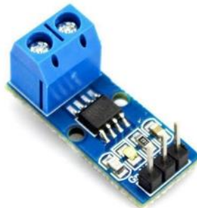
Figure 2: ACS712 Current Sensor
