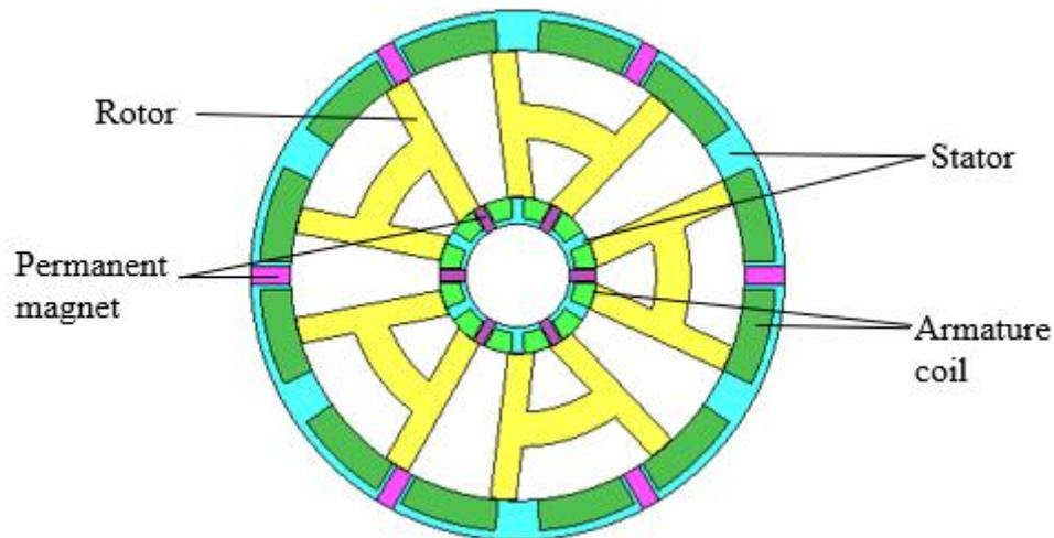
**Figure 3: The design of Double Stator with H-configuration modular rotor PMFSM**
