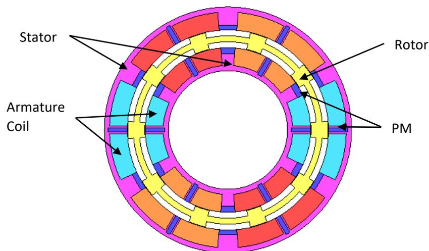
**Figure 1: Conventional design of DS-PMFSM**
