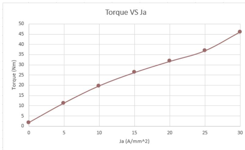
Figure 6: Torque versus current density
