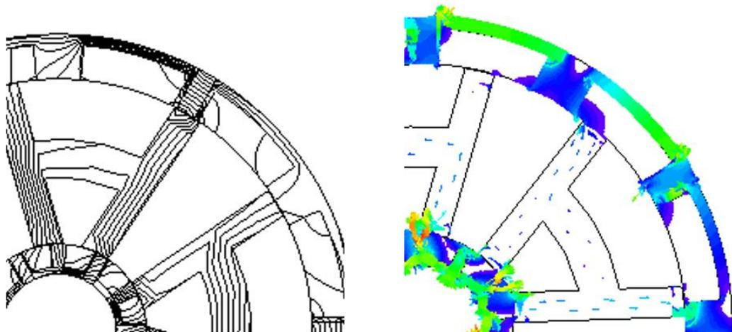
Figure 5: (a) Flux Line of the motor (b) Flux Distribution
