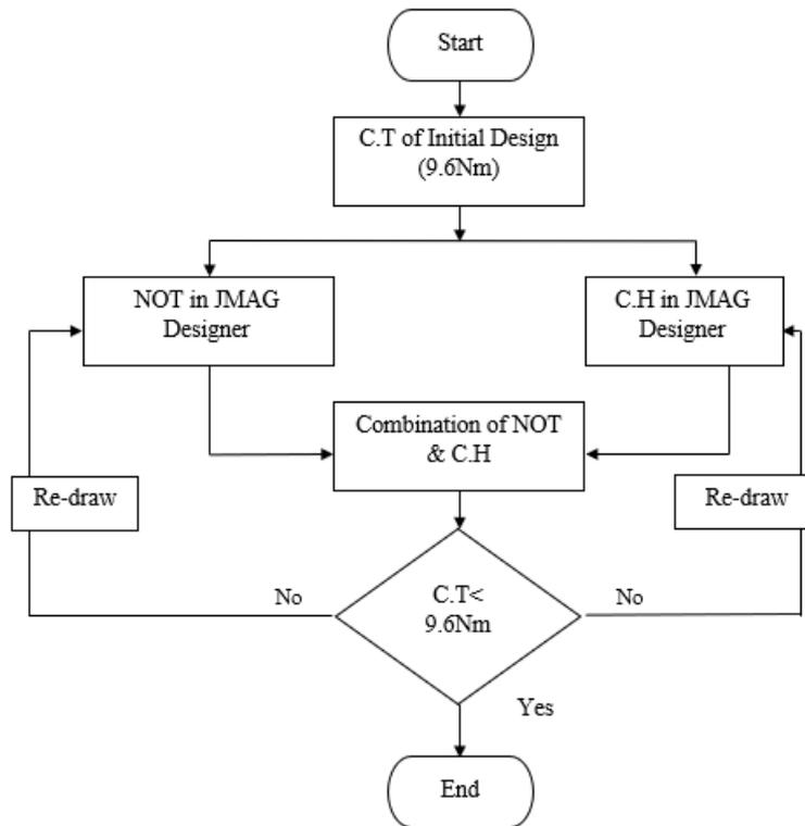
Figure 7: Flow diagram of combined NOT & C.H Technique
