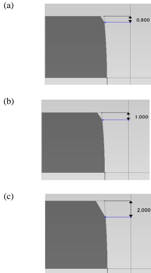
Figure 3: Variation of chamfering at the rotor
