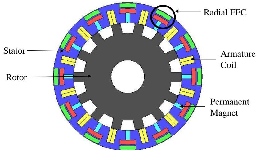
**Figure 1: Initial design of 12S-14P HEFSM**
