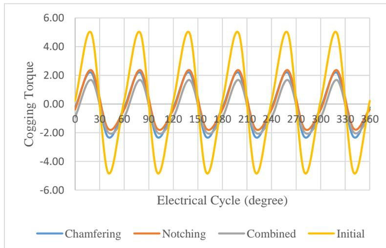
**Figure 11: Waveform of cogging torque combination notching and chamfering**
