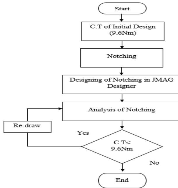
**Figure 5: Flowchart for the notching**
