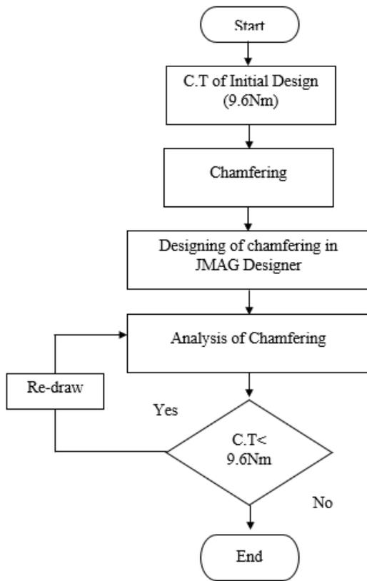
Figure 2: Flowchart of Chamfering
