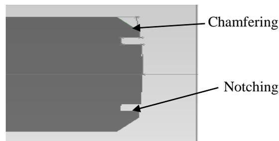
**Figure 6: Combined NOT and C.H design of rotor**
