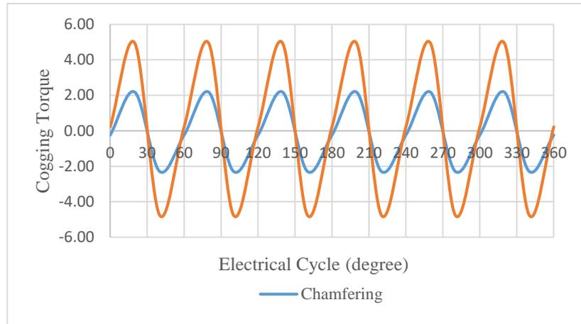
**Figure 9: Waveform of Cogging Torque using Chamfering technique**
