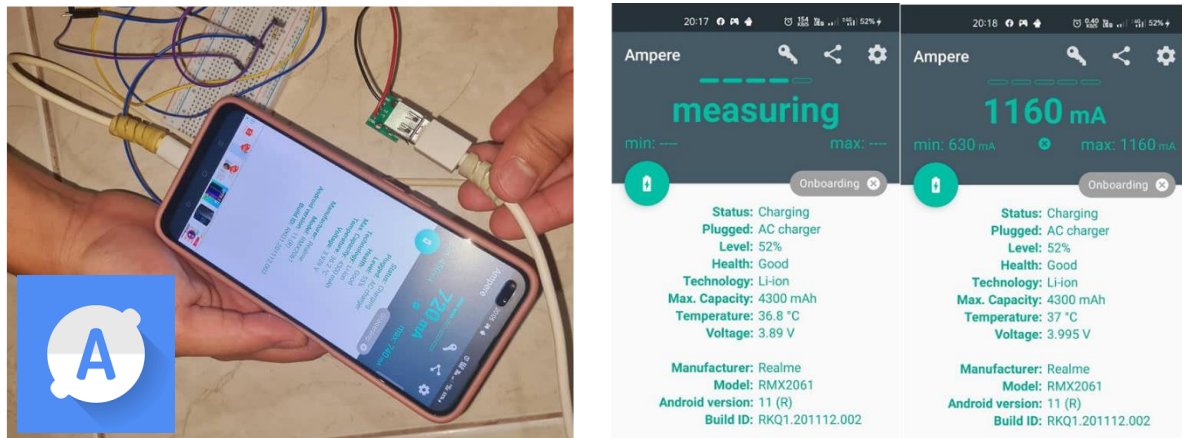
Figure 9: Ampere Apps measuring current from the 18650 Lithium Battery Integrated Module to the mobile phone
