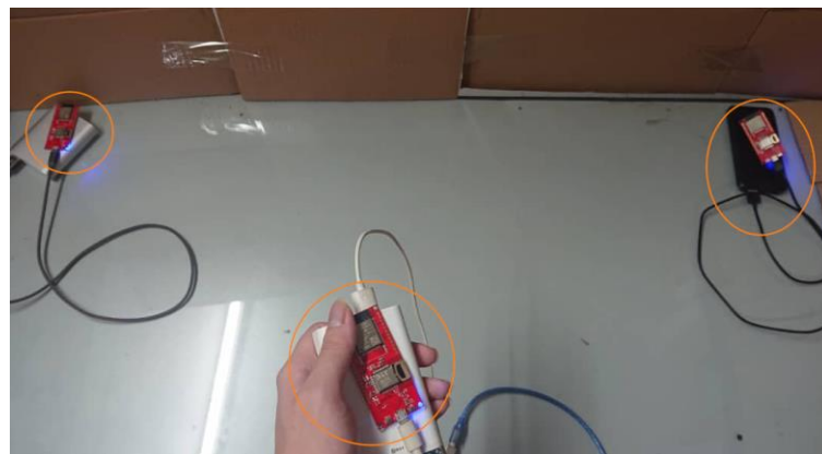
Figure 13: Working of Anchors and Tag
