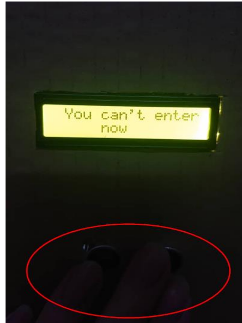
Figure 8: Trying open the door after max. occupancy
