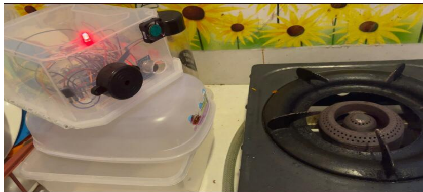
Figure 7: Prototype reacted to LPG above 800 ppm.
