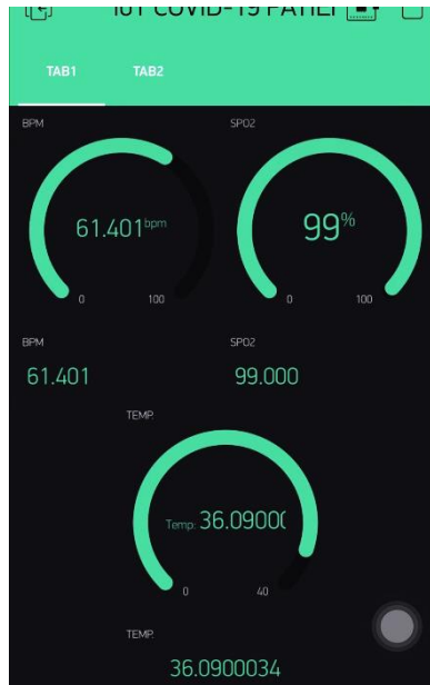
Figure 3: Real-time monitoring method through Blynk application from smartphone
